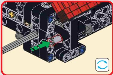
(光滑栓)(Technic Pin without Friction)
